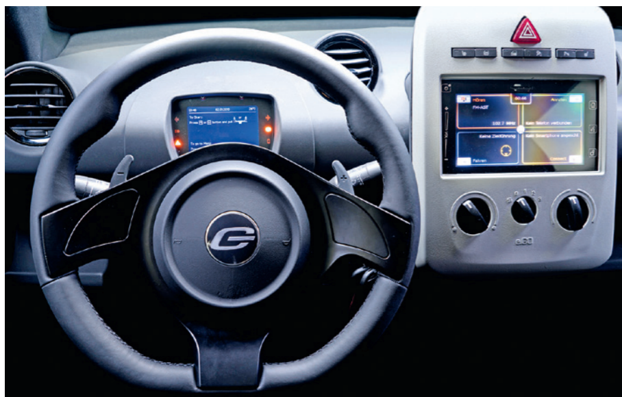
Photo on top: Additive Manufacturing has played a key role in constructing the prototypes. The light-gray section of the dashboard was 3D-printed, for example.
